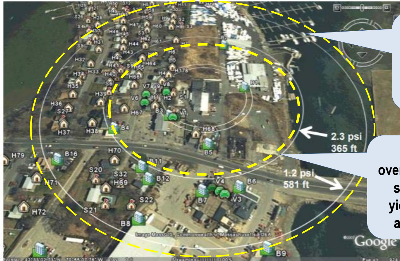
REPORT NO. 2007-03-I-MA , US Chemical Safety Board, Figure 20. Aerial View showing estimated explosion overpressures
